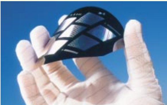
Fig. 1: Highly efficient solar cells on an extremely thin and flexible wafer (40 µm thick). The cells were produced with the LFC (laser-fired contacts) technique, an economic production method which permits very high efficiency values even on thin wafers (20 % for this example).
