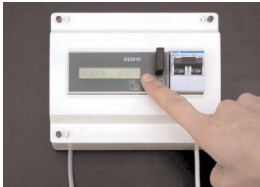
Fig. 1: The "Energy Dispenser" guarantees a certain amount of electricity each day, depending on the tariff class. Up to a certain limit, electricity that the user has not consumed is recorded as a bonus. If plenty of energy is available to the system (e.g. during long sunny periods), the customers can consume twice as much energy for the same price. In the opposite case (e.g. during the night, when the battery is almost flat), only half as much electricity is delivered for the same price. Further flexibility is offered by an electronic key, which "opens up" the energy bonus and can also be used in other households.
