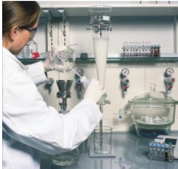
Fig. 1: Testing the disinfection and desalination performance of decentralised systems for drinking water purification.
