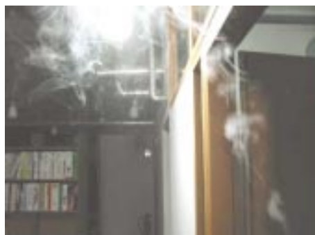
Fig. 2: Visualisation of air currents in a room to check the air exchange in buildings.
