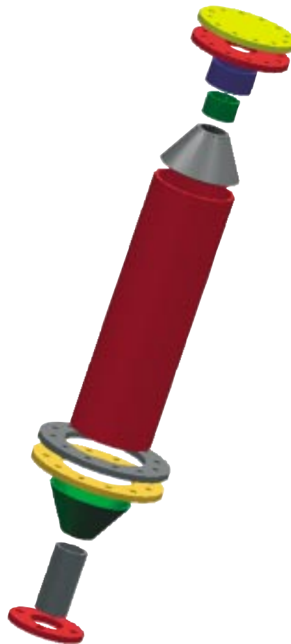
Fig. 1: Exploded view of the reactor, with the inlet at the top and the outlet at the bottom. The reactor honeycomb is not shown. The reactor pipe has a diameter of 124 mm and a length of 400 mm.
