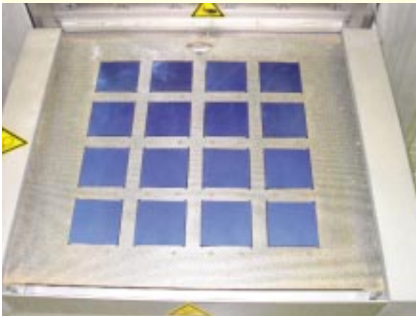
Fig. 1: These wafers were coated with an anti-reflective layer of silicon nitride in our in-line sputtering unit. This technology allows a particularly homogeneous distribution of the coating thickness over large areas. The unit was developed in co-operation with the Applied Films company in Alzenau.
