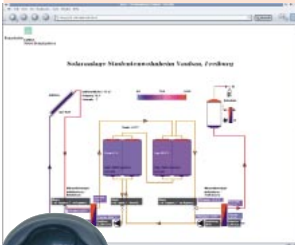
Fig. 1: Internet-based communications concept for a large thermal solar system: Embedded systems provide access to the system state parameters from any location. Meteorological data from the Internet are transferred here using the XML-RPC protocol (via TCP/IP).
