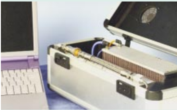
Fig. 1: Fuel-cell power supply for portable electronic appliances. The metal hydride storage unit with 250 NI hydrogen is located in the front of the box at the right of the photo. Behind it is the fuel-cell stack with a peak power exceeding 100 W.
