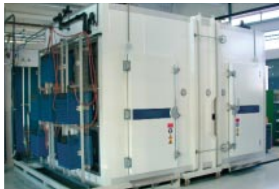
Fig. 2: Double climatic chamber to test windows, solar facades and solar modules at Fraunhofer ISE. The effect of temperature or humidity gradients across the building envelope can be tested in the chamber under controlled and accelerated conditions.
