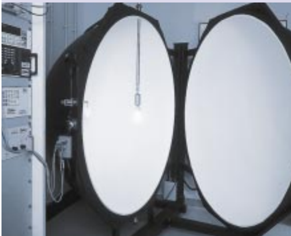
Fig. 1: Integrating-sphere photometer to measure the luminous flux of DC lamps and light sources.
