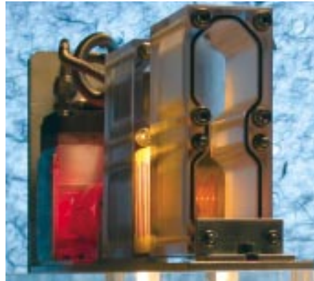
Fig. 1: Complete system including an electrolyser unit to supply gas to gasochromic windows. In the foreground is the electrolyser unit (yellow) and the transparent tank housing (70 mm x 120 mm x 40 mm). Behind them is the pump (red/silver).
