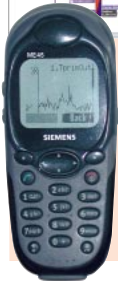
Fig. 2: The GSM-Wap interface allows remote access to system operation via a mobile phone. If a fault occurs, the control system sends a signal with SMS (short message service).
