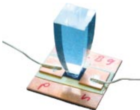
Fig. 1: Two-stage photovoltaic concentrator system. Despite single-axis tracking, a geometric concentration factor exceeding 300 is achieved. The second concentrator stage (compound parabolic concentrator - CPC) adheres directly to the silicon concentrator cells, that were developed specifically for this purpose (see photo). The cells, each with an area of only 4.5 mm x 4.5 mm, have an efficiency value of 24 % for an illumination of 100 suns.
